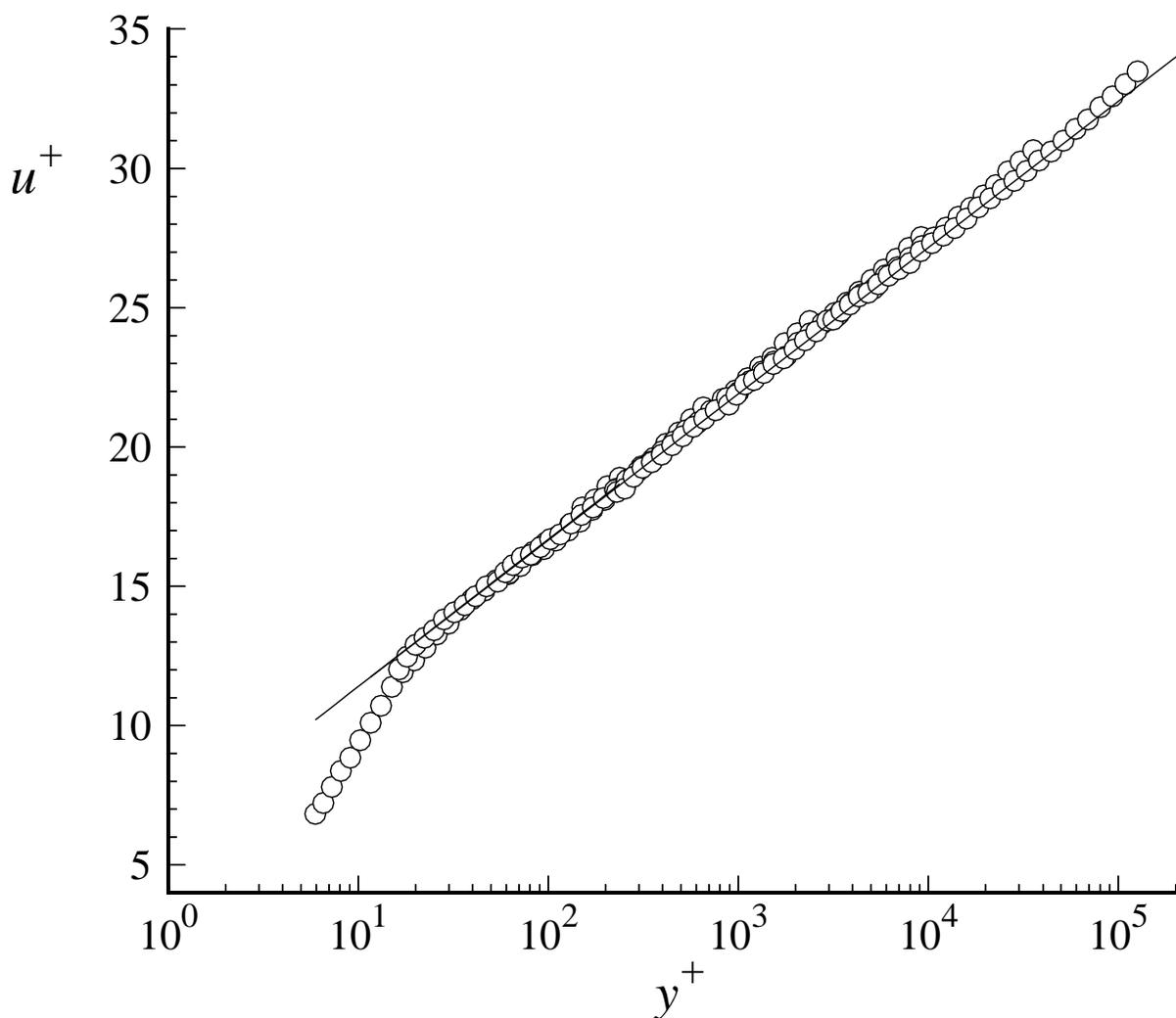
Figure 7.21: Mean velocity profiles in fully-developed turbulent pipe flow. Symbols, experimental data of Zagarola and Smits (1997) for  $y/R < 0.1$ , for the same values of  $Re$  as in Fig. 7.20. Line, log law with  $\kappa = 0.436$  and  $B = 6.13$ .
