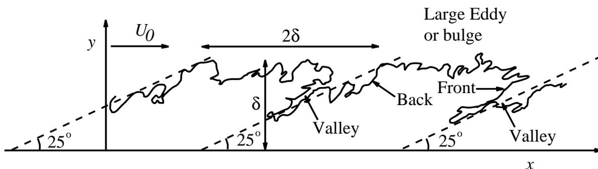
Figure 7.44: The large-scale features of a turbulent boundary layer at  $Re_\theta \approx 4,000$ . The irregular line—approximating the viscous superlayer—is the boundary between smoke-filled turbulent fluid and clear free-stream fluid. (From the experiment of Falco 1977.)
