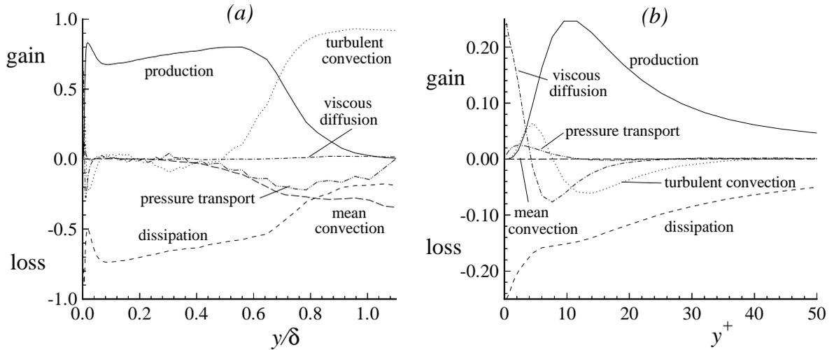
Figure 7.34: Turbulent kinetic energy budget in a turbulent boundary layer at  $Re_\theta = 1,410$ : terms in Eq. (7.177) (a) normalized as a function of  $y$  so that the sum of the squares of the terms is unity (b) normalized by the viscous scales. From the DNS data of Spalart (1988).
