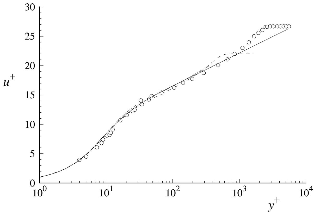
Figure 7.27: Mean velocity profiles in wall units. Circles, boundary-layer experiments of Klebanoff (1954),  $Re_\theta = 8,000$ ; dashed line, boundary-layer DNS of Spalart (1988),  $Re_\theta = 1,410$ ; dot-dashed line, channel flow DNS of Kim *et al.* (1987),  $Re = 13,750$ ; solid line, van Driest's law of the wall, Eqs. (7.144)–(7.145).
