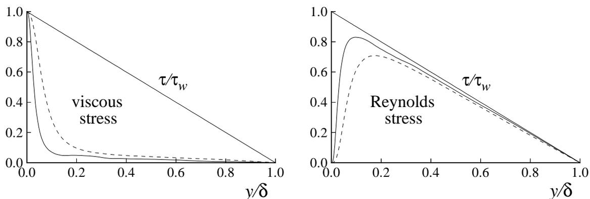
Figure 7.3: Profiles of the viscous shear stress, and the Reynolds shear stress in turbulent channel flow: DNS data of Kim *et al.* (1987): dashed line,  $Re = 5,600$ ; solid line,  $Re = 13,750$ .
