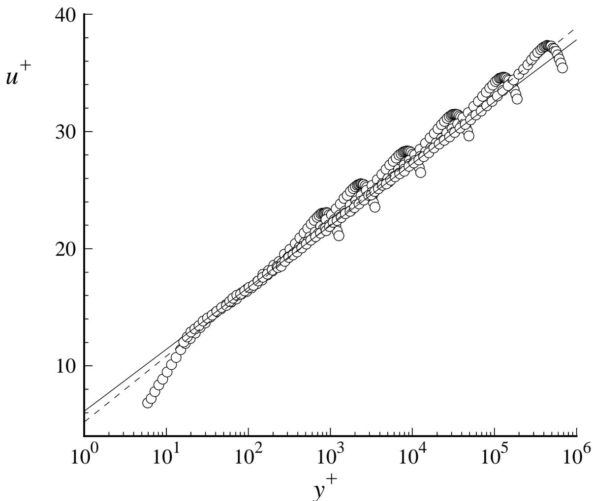
Figure 7.20: Mean velocity profiles in fully-developed turbulent pipe flow. Symbols, experimental data of Zagarola and Smits (1997) at six Reynolds numbers ( $Re \approx 32 \times 10^3$ ,  $99 \times 10^3$ ,  $409 \times 10^3$ ,  $1.79 \times 10^6$ ,  $7.71 \times 10^6$ ,  $29.9 \times 10^6$ ). Solid line, log law with  $\kappa = 0.436$  and  $B = 6.13$ ; dashed line, log law with  $\kappa = 0.41$ ,  $B = 5.2$ .
