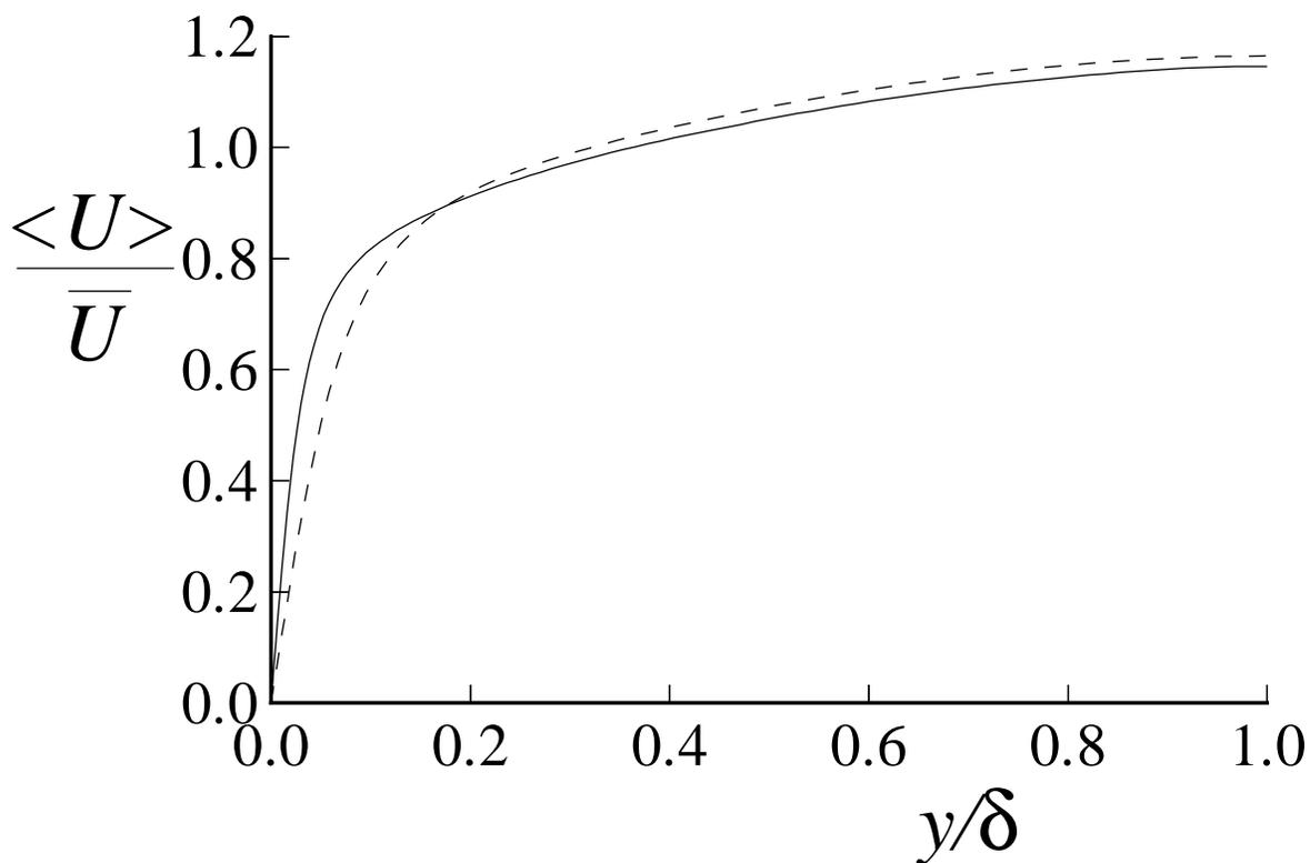
Figure 7.2: Mean velocity profiles in fully-developed turbulent channel flow from the DNS of Kim *et al.* (1987): dashed line,  $Re = 5,600$ ; solid line,  $Re = 13,750$
