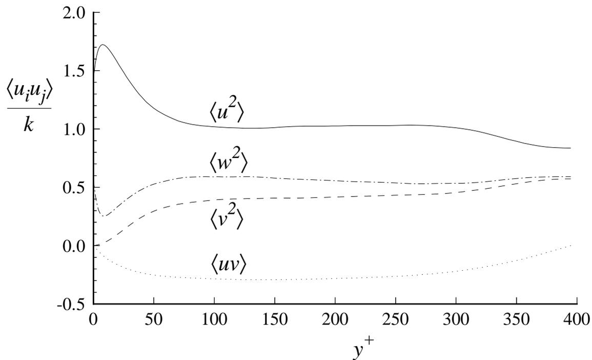
Figure 7.15: Profiles of Reynolds stresses normalized by turbulent kinetic energy from DNS of channel flow at  $\text{Re} = 13,750$  (Kim *et al.* 1987).
