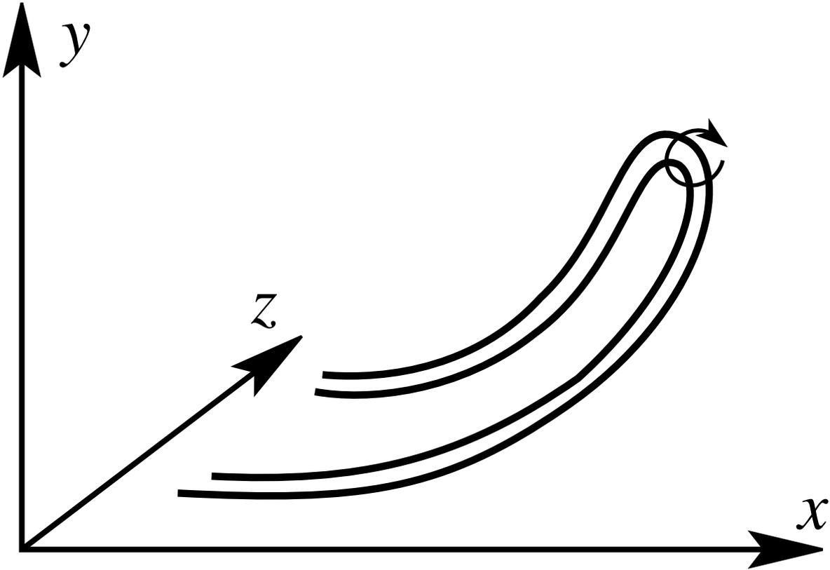
Figure 7.43: Sketch of counter-rotating rolls in the near-wall region. (From Holmes *et al.* 1996.)
