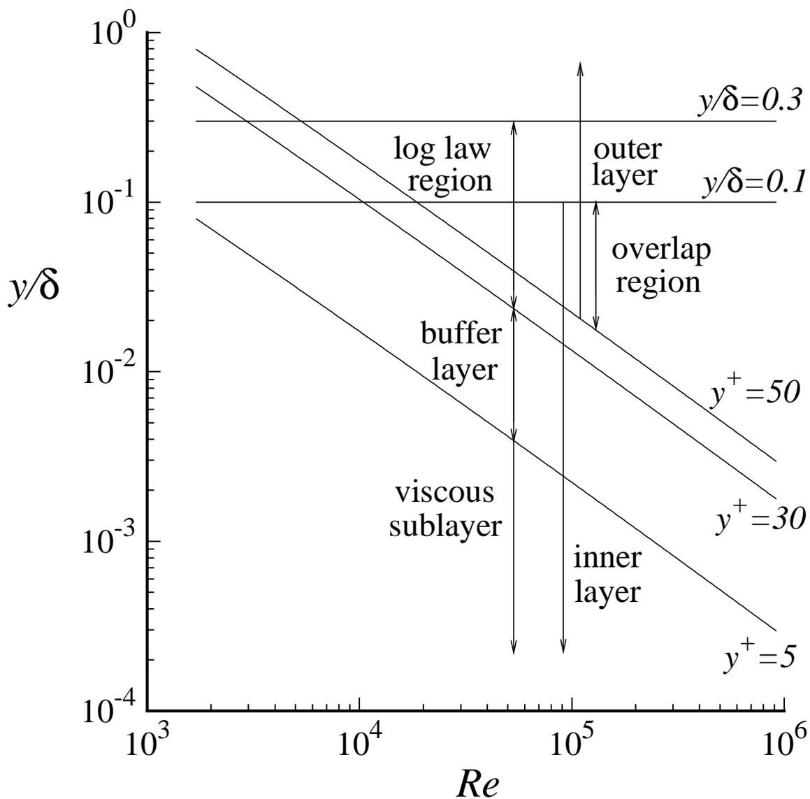
Figure 7.13: Regions and layers in turbulent channel flow as functions of Reynolds number.
