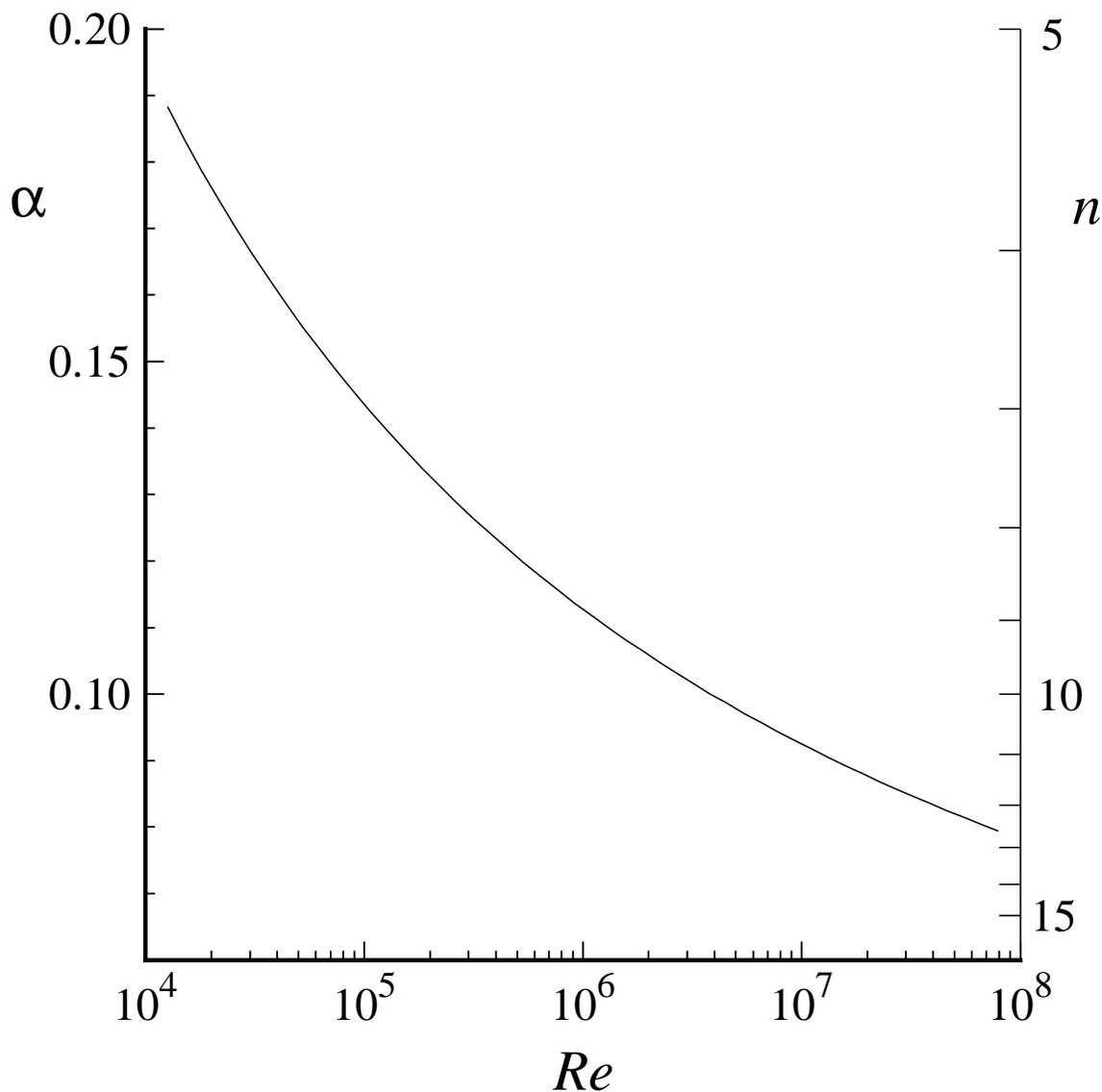
Figure 7.32: Exponent  $\alpha = 1/n$  (Eq. 7.158) in the power-law  $u^+ = C(y^+)^\alpha = C(y^+)^{1/n}$  for pipe flow as a function of Reynolds number.
