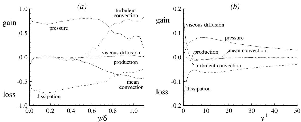
Figure 7.37: Budget of  $\langle w^2 \rangle$  in a turbulent boundary layer: conditions and normalization are the same as in Fig. 7.34.
