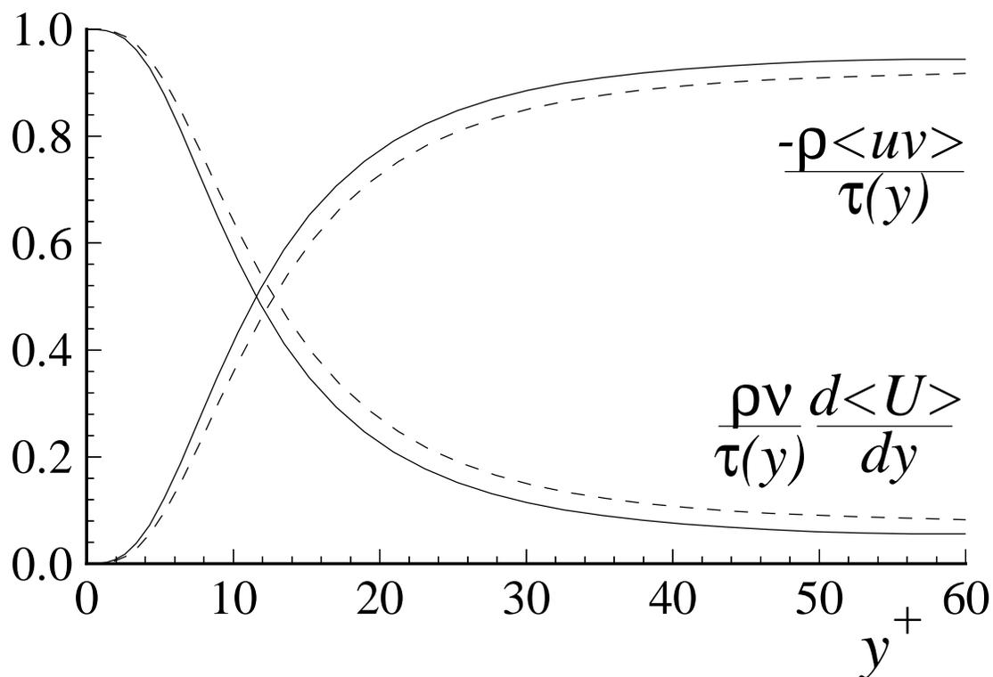
Figure 7.4: Profiles of the fractional contributions of the viscous and Reynolds stresses to the total stress. DNS data of Kim *et al.* (1987): dashed lines,  $Re = 5,600$ ; solid lines,  $Re = 13,750$ .
