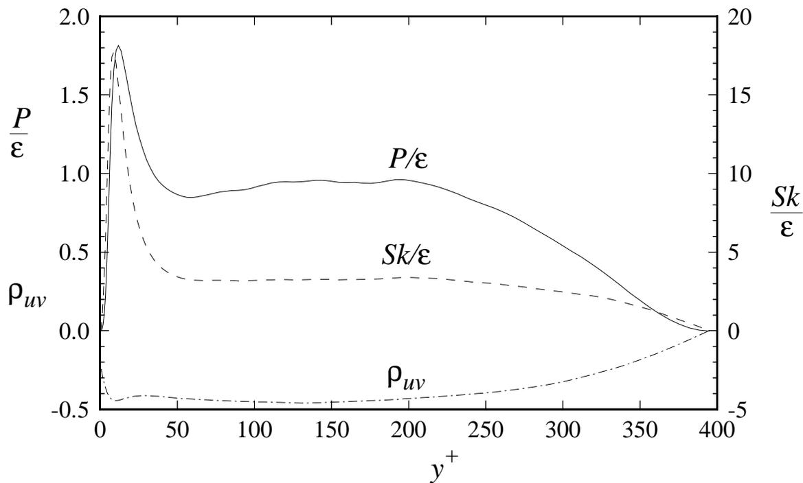
Figure 7.16: Profiles of the ratio of production to dissipation ( $\mathcal{P}/\epsilon$ ), normalized mean shear rate ( $\mathcal{S}k/\epsilon$ ), and shear stress correlation coefficient ( $\rho_{uv}$ ) from DNS of channel flow at  $\text{Re} = 13,750$  (Kim *et al.* 1987).
