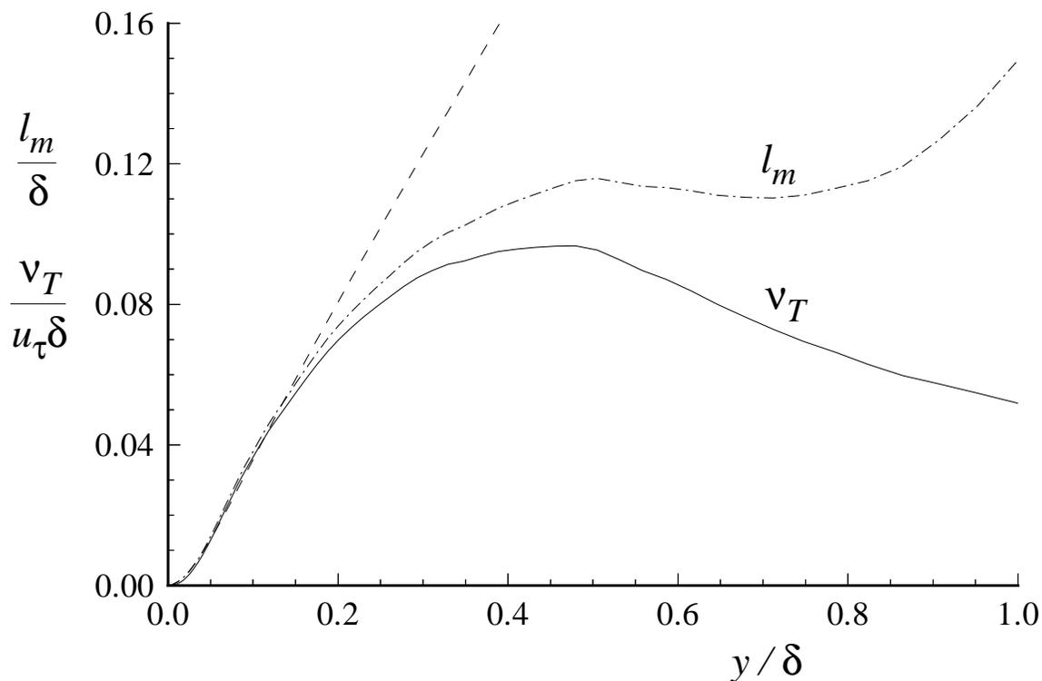
Figure 7.30: Turbulent viscosity and mixing length deduced from direct numerical simulations of a turbulent boundary layer (Spalart 1988). Solid line,  $\nu_T$  from DNS; dot-dash line,  $l_m$  from DNS; dashed line  $l_m$  and  $\nu_T$  according to van Driest's specification (Eq. 7.145).
