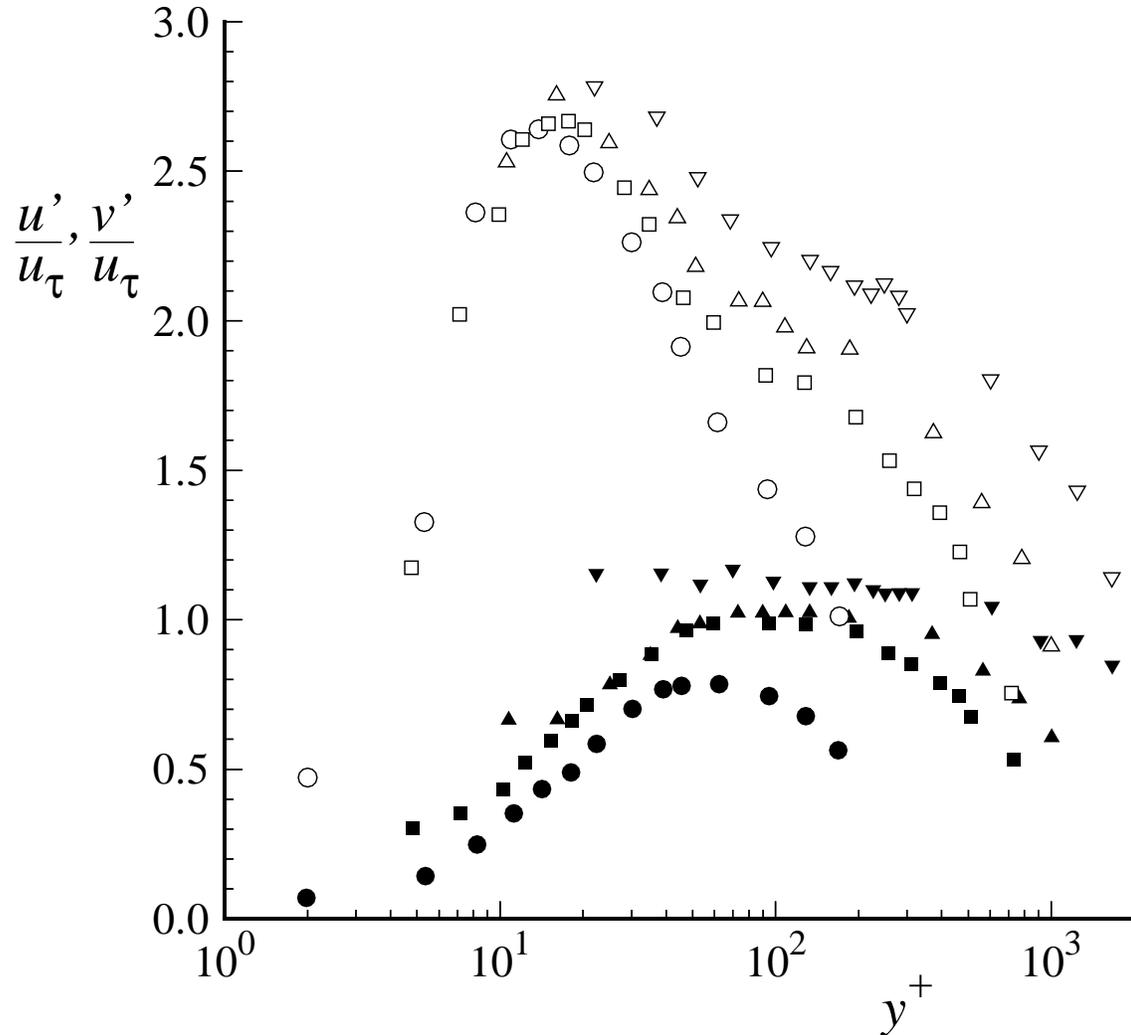
Figure 7.19: Profiles of r.m.s. velocity measured in channel flow at different Reynolds numbers by Wei and Willmarth (1989). Open symbols:  $u'/u_\tau = \langle u^2 \rangle^{1/2}/u_\tau$ ;  $\circ$ ,  $Re_0 = 2,970$ ;  $\square$ ,  $Re_0 = 14,914$ ;  $\triangle$ ,  $Re_0 = 22,776$ ;  $\nabla$ ,  $Re_0 = 39,582$ . Solid symbols:  $v'/u_\tau = \langle v^2 \rangle^{1/2}/u_\tau$  at the same Reynolds numbers.
