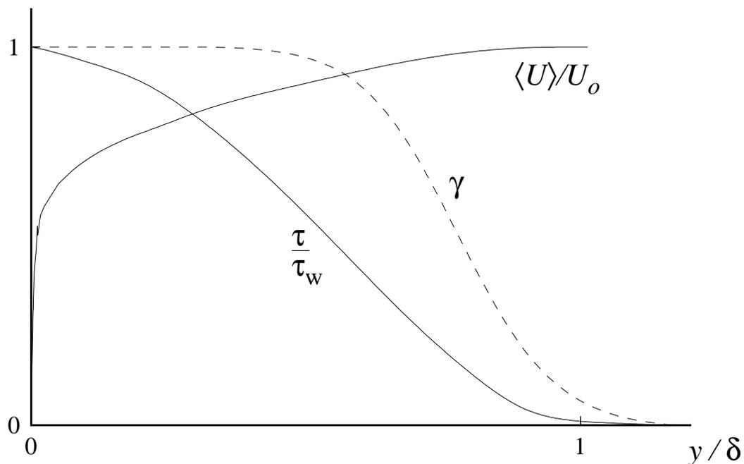
Figure 7.26: Profiles of mean velocity, shear stress and intermittency factor in a zero-pressure gradient turbulent boundary layer,  $Re_\theta = 8,000$ . From the experimental data of Klebanoff (1954).
