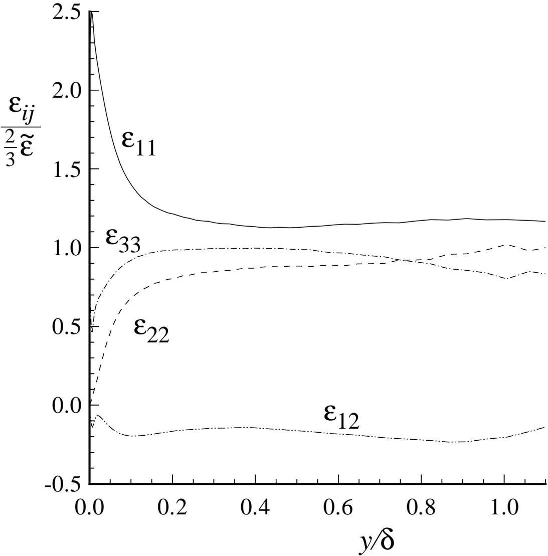
Figure 7.39: Normalized dissipation components in a turbulent boundary layer at  $Re_\theta = 1,410$ : from the DNS data of Spalart (1988) for which  $\delta = 650\delta_\nu$ .
