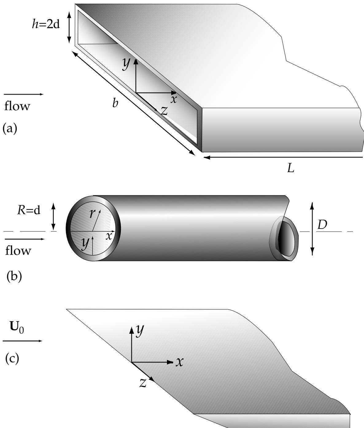
Figure 7.1: Sketch of (a) channel flow (b) pipe flow and (c) flat-plate boundary layer.
