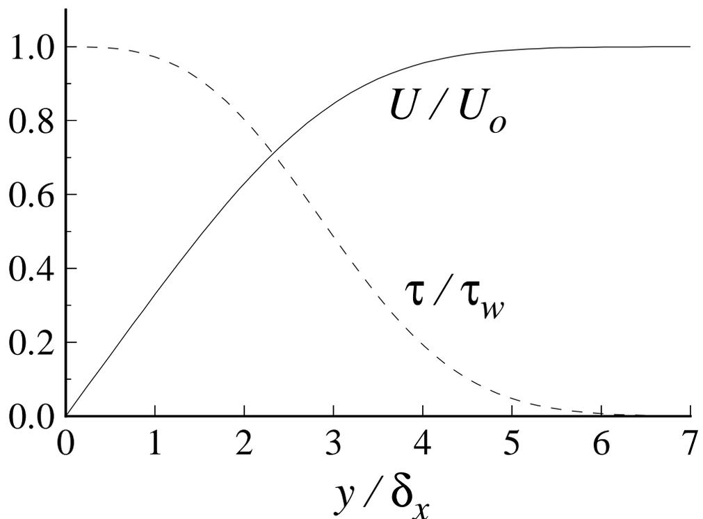
Figure 7.25: Normalized velocity and shear stress profiles from the Blasius solution for the zero-pressure-gradient laminar boundary layer on a flat plate:  $y$  is normalized by  $\delta_x \equiv x/\text{Re}_x^{1/2} = (x\nu/U_0)^{1/2}$ .
