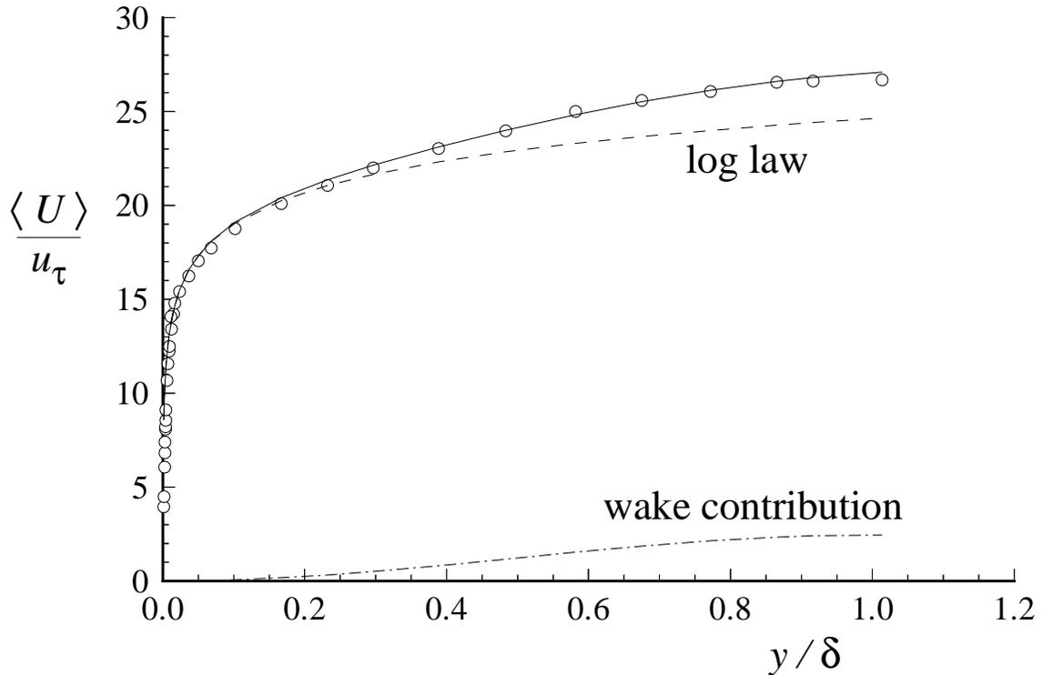
Figure 7.28: Mean velocity profile in a turbulent boundary layer showing the law of the wake. Symbols, experimental data of Klebanoff (1954); dashed line, log law ( $\kappa = 0.41$ ,  $B = 5.2$ ); dot-dashed line, wake contribution  $\Pi w(y/\delta)/\kappa$  ( $\Pi = 0.5$ ); solid line, sum of log law and wake contribution (Eq. 7.148).
