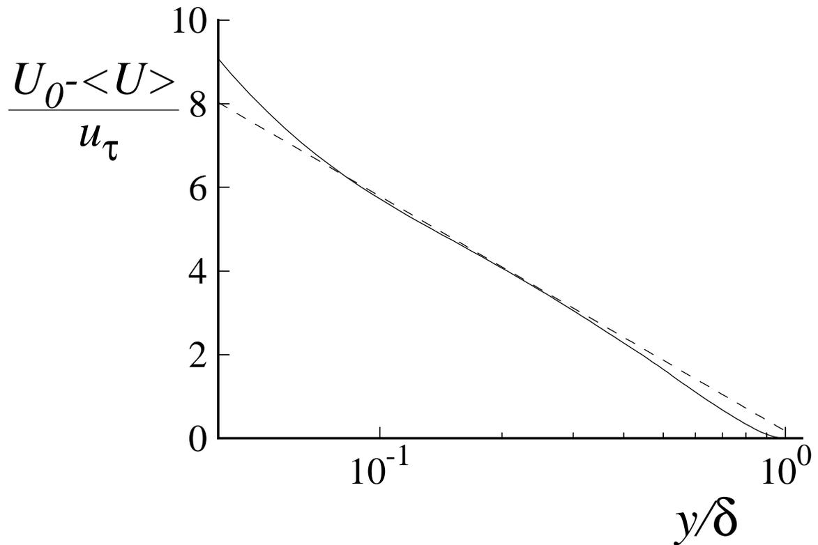
Figure 7.9: Mean velocity defect in turbulent channel flow. Solid line, DNS of Kim *et al.* (1987),  $Re = 13,750$ ; dashed line, log law, Eqs. (7.43)–(7.44).
