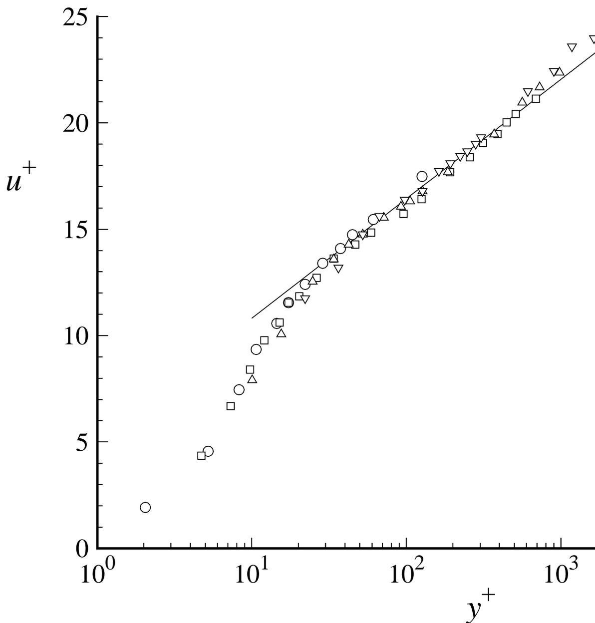
Figure 7.7: Mean velocity profiles in fully-developed turbulent channel flow measured by Wei and Willmarth (1989):  $\circ$ ,  $Re_0 = 2,970$ ;  $\square$ ,  $Re_0 = 14,914$ ;  $\triangle$ ,  $Re_0 = 22,776$ ;  $\nabla$ ,  $Re_0 = 39,582$ ; line, the log law, Eqs. (7.43)–(7.44).
