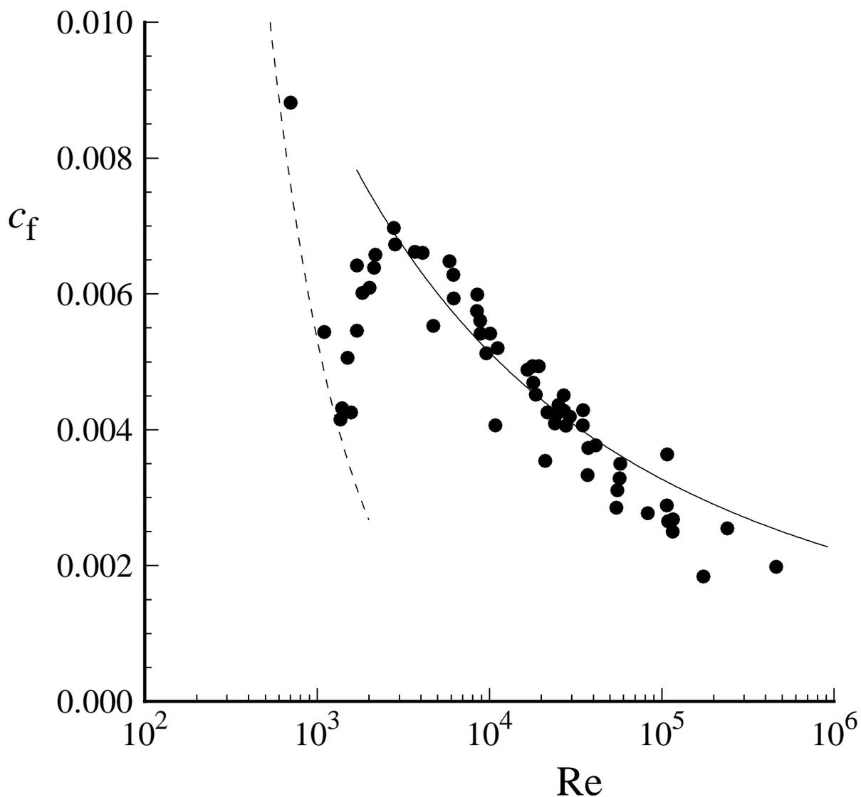
Figure 7.10: Skin friction coefficient  $c_f \equiv \tau_w / (\frac{1}{2}\rho U_0^2)$  against Reynolds number ( $Re = 2\bar{U}\delta/\nu$ ) for channel flow: symbols, experimental data compiled by Dean (1978); solid line, from Eq. (7.55); dashed line, laminar friction law  $c_f = 16/(3Re)$ .
