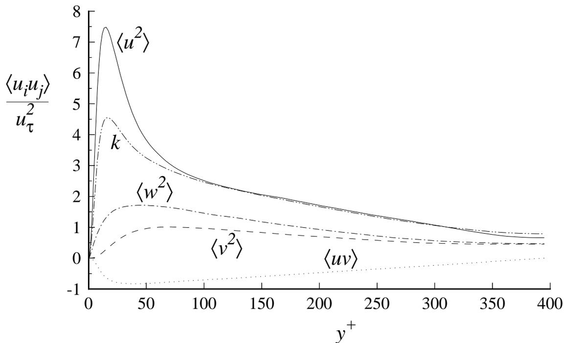
Figure 7.14: Reynolds stresses and kinetic energy normalized by friction velocity against  $y^+$  from DNS of channel flow at  $\text{Re} = 13,750$  (Kim *et al.* 1987).
