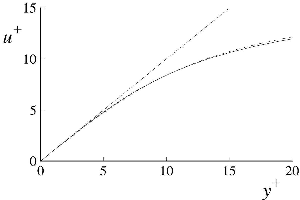
Figure 7.5: Near-wall profiles of mean velocity from the DNS data of Kim *et al.*: dashed line,  $Re = 5,600$ ; solid line,  $Re = 13,750$ ; dot-dashed line,  $u^+ = y^+$ .
