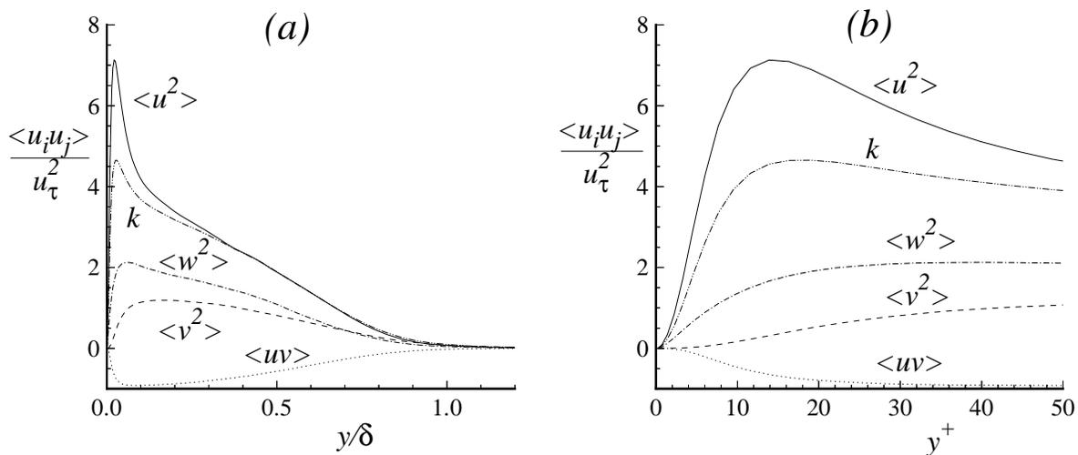
Figure 7.33: Profiles of Reynolds stresses and kinetic energy normalized by the friction velocity in a turbulent boundary layer at  $\text{Re}_\theta = 1,410$ : (a) across the boundary layer (b) in the viscous near-wall region. From the DNS data of Spalart (1988).
