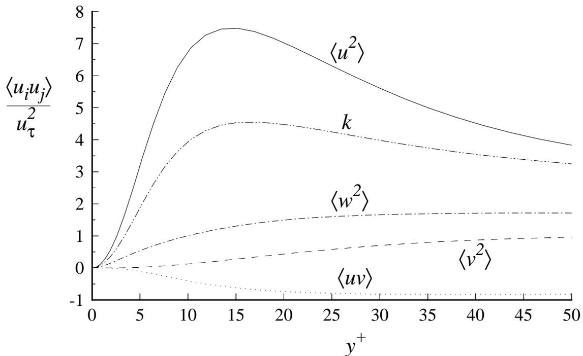
Figure 7.17: Profiles of Reynolds stresses and kinetic energy normalized by friction velocity in the viscous wall region of turbulent channel flow: DNS data of Kim *et al.* (1987)  $Re = 13,750$ .
