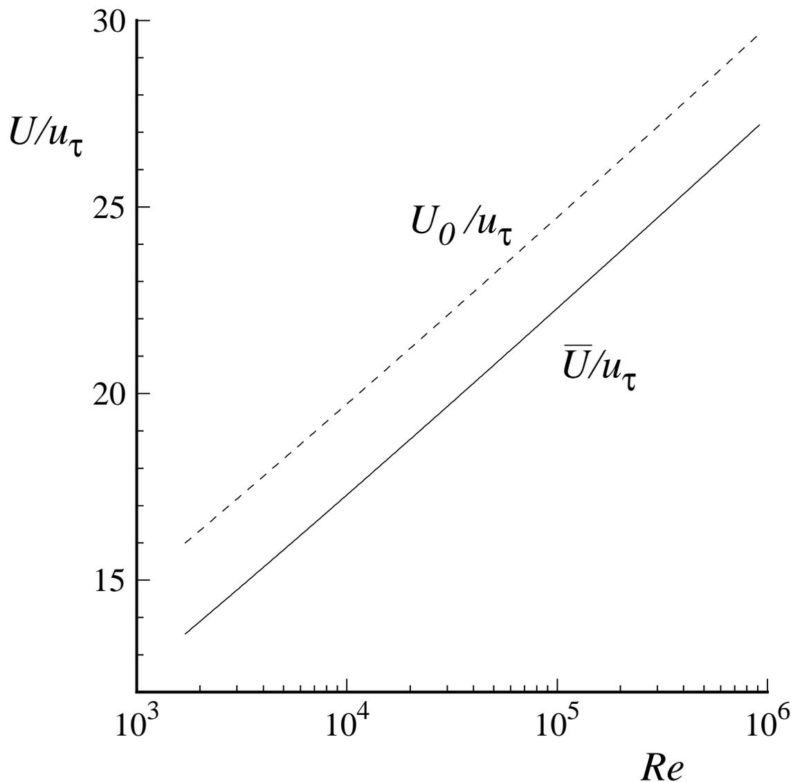
Figure 7.12: Outer-to-inner velocity scale ratios for turbulent channel flow as functions of Reynolds number (obtained from Eq. 7.55): solid line,  $\bar{U}/u_\tau$ ; dashed line  $U_0/u_\tau$ .
