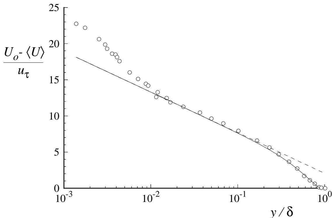
Figure 7.29: Velocity defect law. Symbols, experimental data of Klebanoff (1954); dashed line, log law; solid line, sum of log law and wake contribution  $\Pi w(y/\delta)/\kappa$ .
