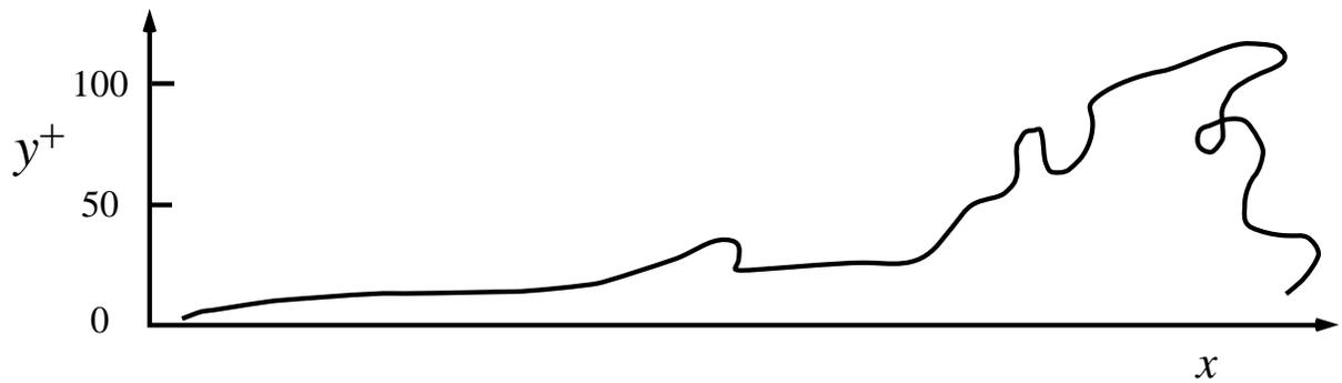
Figure 7.40: Dye streak in a turbulent boundary layer showing the ejection of low-speed near-wall fluid. (From the experiment of Kline *et al.* 1967.)
